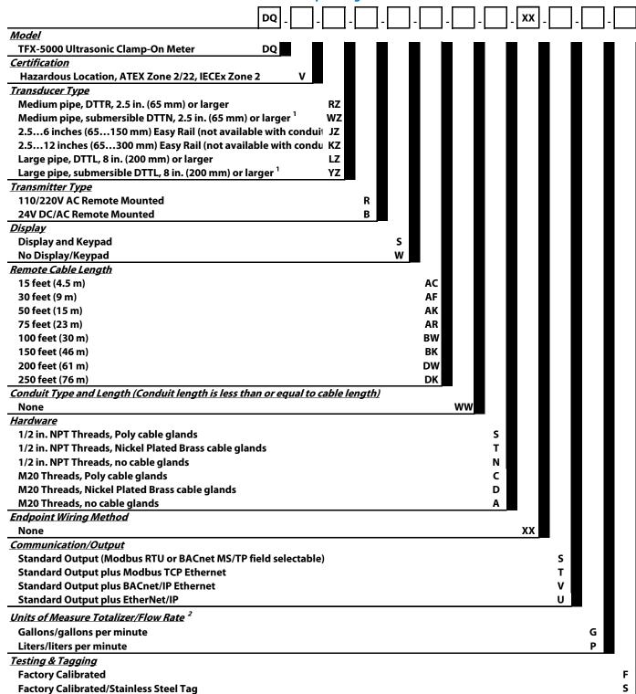
Part Number Construction for TFX-5000 Flow Meters for Pipes Larger than 2 in. for ATEX/IECEx Hazardous Locations
