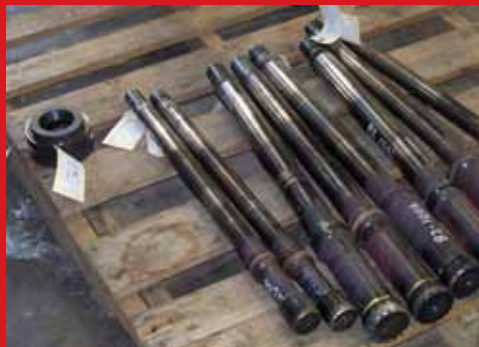
Valtek® 6" Channel Stream Pressure Balanced Plug & Stem Assembly, Multi Stage Retainer and Sleeve
